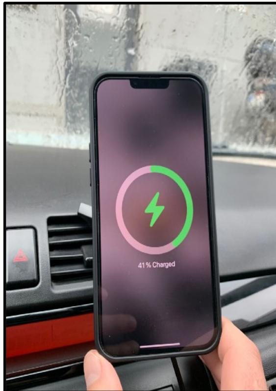
3. To remove the phone, simply pull it away from the magnetic surface.
