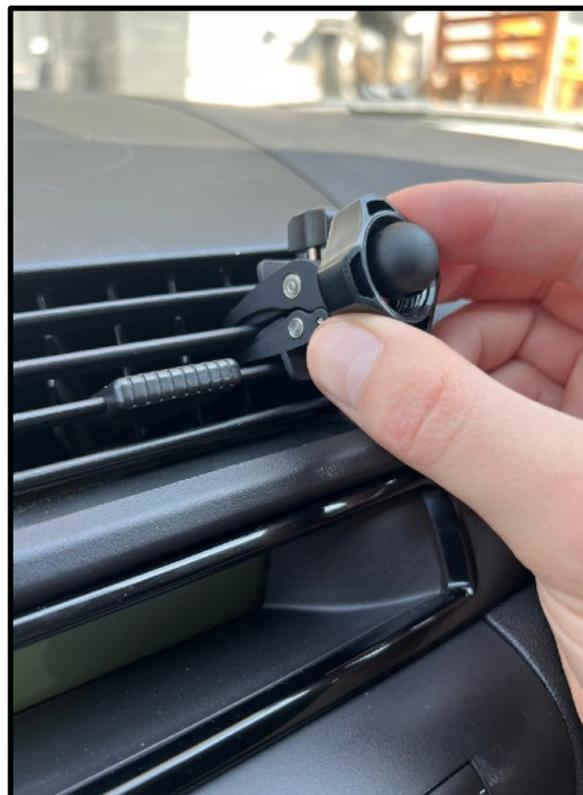
4. Slide the rear of the bracket with the magnetic surface into the plastic nut, then screw the nut in until the connection is tight.
