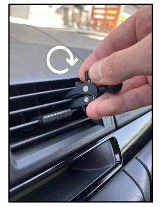
3. Install the plastic nut on the front of the bracket.
